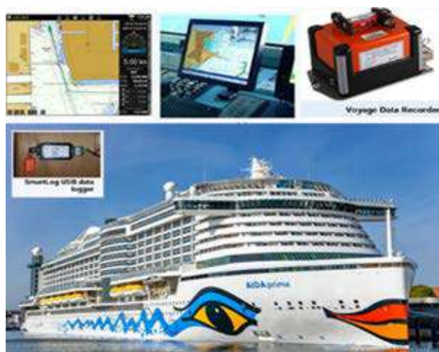
Figure 3: Example of standard navigation instruments that can be used to collect CSB data through a logger
