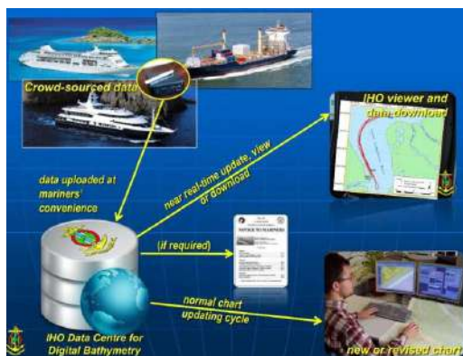
Figure 5: CSB Data and IHODCDB Workflow (CSBWG,2022)
